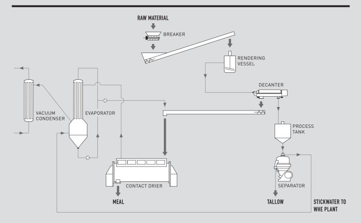
The Rendertech Centrifuge Dewatering System (CDS) is a low-temperature wet rendering process suitable for plant raw material capacities up to 10 tonne/hr.
