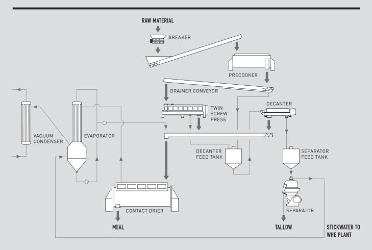
The Rendertech Press Dewatering System (PDS) is a low-temperature wet rendering process suitable for plant raw material capacities of 5 tonne/hr and above.
