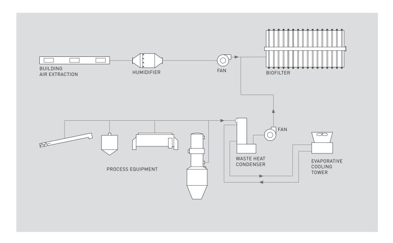
Rendering plants require a comprehensive odour control system to ensure they meet regulatory requirements. A Rendertech Odour Control System captures odorous vapours at their source and removes them for treatment. Our design engineers consider the full odour control system and, as necessary, will supply correctly sized ducting, fans, condensers, hot water tanks, and evaporative cooling towers, as well as humidifiers and biofilters.
