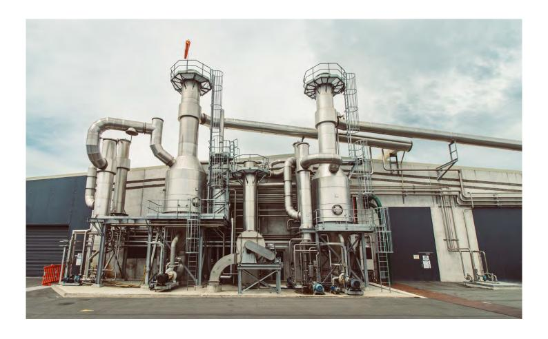
A Rendertech Evaporator is a shell-and-tube heat exchanger that uses heat from water vapour or steam to evaporate water in order to concentrate a solution or slurry. In a rendering plant, Evaporator plants can be used to recover valuable products from liquid waste streams or to thicken a product slurry before it is cooked or dried.
