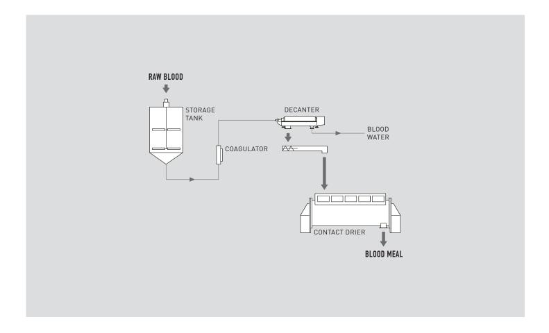
The Rendertech Blood Processing System (BPS) is a continuous process for converting animal blood into a high-quality blood meal. The process is efficient, economical, and simple to operate, with the key piece of process equipment being the steam-heated Rendertech Contact Drier (CD).
