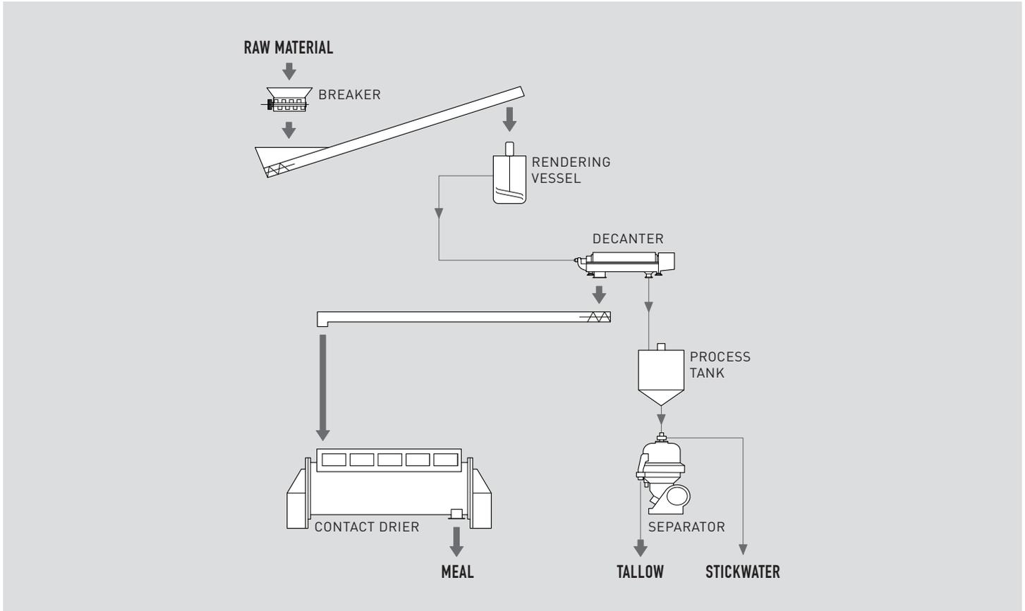
The Rendertech Centrifuge Dewatering System (CDS) is a low-temperature wet rendering process suitable for plant raw material capacities up to 8 tonnes/hr. The system produces quality products, has low energy consumption, and is simple to operate. The compact, versatile plant can process a wide range of raw materials. When fitted with a Rendertech Waste Heat Evaporator for stickwater recovery, the process is virtually 'zero waste', resulting in high product yield and low wastewater loads.
