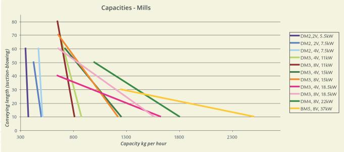
5.5/2 to be read: 5.5 kW with 2 fan wings etc.
