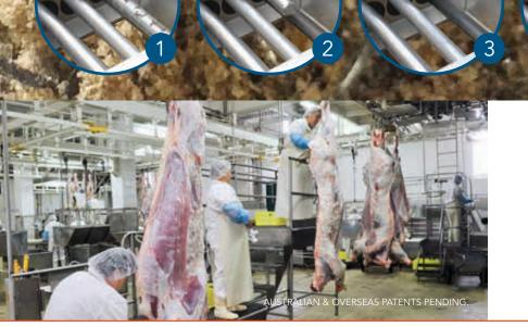
During the process of turning offal into meat meal, small drenching capsule springs left in the animals stomach at the time of slaughter are ground up by mills and grinders, causing metal contamination.
