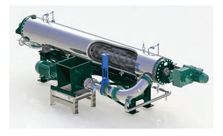
The Rendertech Continuous Feather Hydrolyser converts poultry feathers and hog hair into a highly nutritional animal feed. It is simple to operate and maintain with automated controls. Features include an integrated drainer section in the feeder to remove excess water and thus improve efficiency. The steamheated jacket and direct steam injection produce a consistant finished product.
