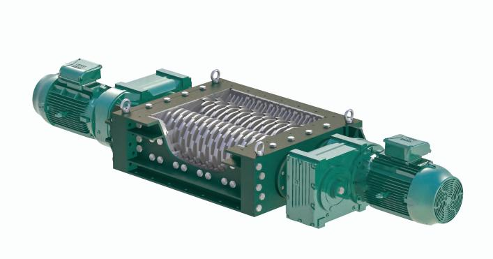
The Rendertech Fine Crusher is a secondary sizing machine following a Breaker. It produces an optimum particle size for most low-temperature rendering systems and for high-temperature continuous dry rendering. The main advantages of a smaller particle size are an increased plant capacity, improved meal quality, lower energy use, and reduced plant maintenance.
