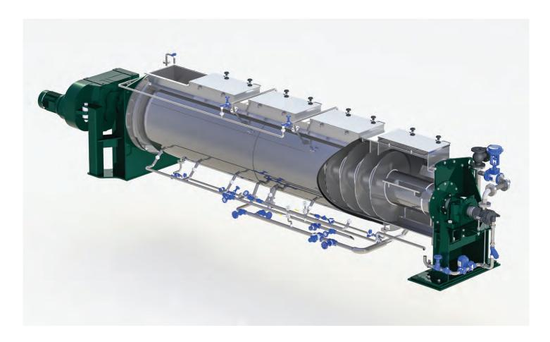
The Rendertech Fish Cooker is an indirect steam cooker used for processing high-yield raw materials. Its gentle screw rotor and even heating action ensure raw material structure is maintained during processing, leading to better pressing and better separation of solids, oil and water. The slow rotation speed makes the process very gentle on raw material.
