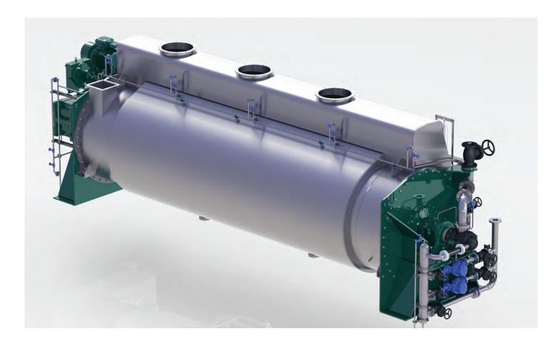
The Rendertech Continuous Cooker is used as part of a continuous high-temperature rendering process. Product is heated indirectly with a series of hollow, steam-heated discs mounted on a central rotating shaft. This design gently heats the product with no harsh agitation to ensure efficient separation of the fat from the cake in subsequent processes.
