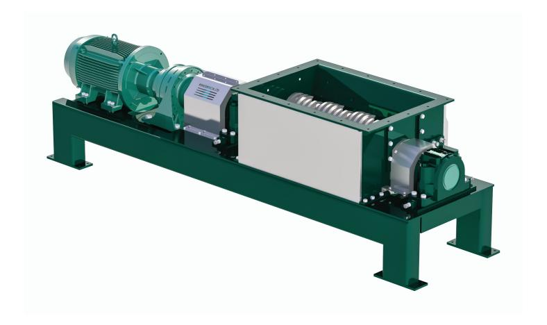
The Rendertech Breaker is a generalpurpose sizing machine for the primary breakdown of raw materials. The design and configuration of the machine allow it to be used as a primary breaker and/or a secondary fine crusher. It is designed to be low speed, high torque, low power, and minimal maintenance compared with most alternative options available on the market.
